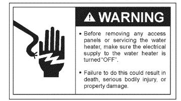
1. Before beginning turn "OFF" the electric power supply to the water heater.
